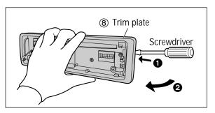
Pull out the unit while pushing down the lock lever with a screwdriver.
